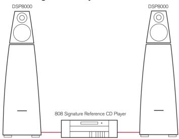
Meridian DSP loudspeakers include DSP volume and tone controls, and be connected directly to digital sources, such as the 808 Signature Reference CD Player, to create an compact high-quality music system.
