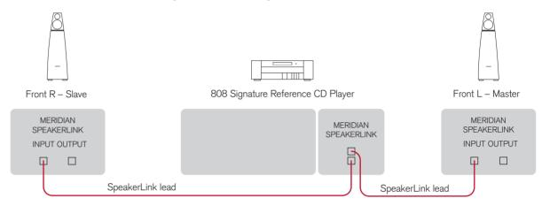
You can create a complete system by connecting a pair of DSP8000 loudspeakers directly to a digital source. The DSP loudspeakers include volume, balance, and tone controls allowing you to control the system using an MSR+.
