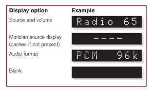
The audio format display shows **PCM**, **Data**, or **MHR**, followed by the frequency or **NL** (not locked).
